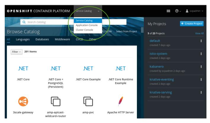
The OpenShift Container Platform includes a *service catalog*, an implementation of the <u>Open Service Broker API</u> (OSB API) for Kubernetes. This allows users to connect any of their applications deployed in OpenShift Container Platform to a wide variety of service brokers.
